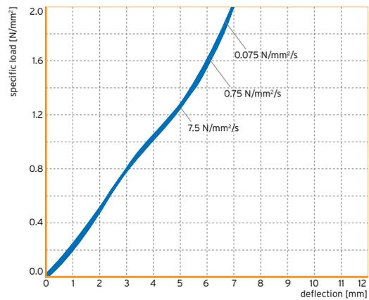
**dependency on amplitude:** preload at static load limit; form factor:  $q=3$ , thickness of material 25 mm
